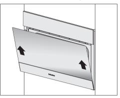
Holding the door evenly with both hands, lift the door up at a slant and off the hinges.
